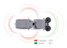
Everything at a glance: The fully glazed comfort cabin offers the driver an excellent view of his surroundings. The camera system extends the driver's field of vision by another 270° – and automatically provides a view to the side when turning.
