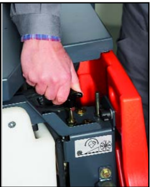
The control for the large dirt flap allows the operator to pick up large items during the course of sweeping.
