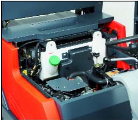
The engine compartment provides easy access for maintenance and service.
