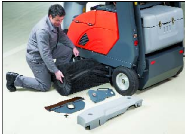
Change-out of main sweeping brush requires no tools and is quick and simple.
